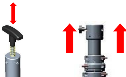
Figure 5-2.1: Use of the pneumatic hand pump
