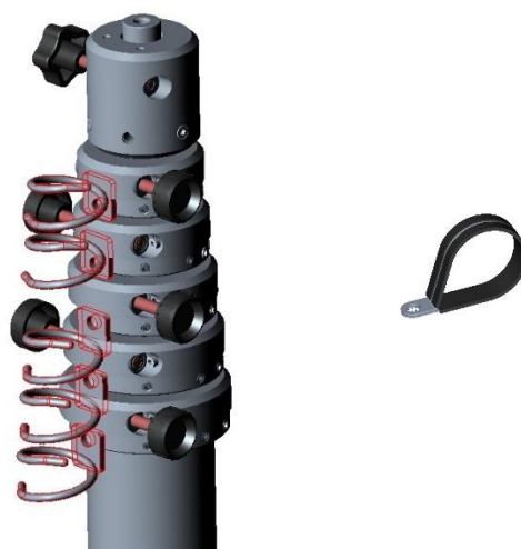
Figure 4-5.7: Helicoidal cable guides (to the left) and simple guiding rings made of rubber (to the right)
