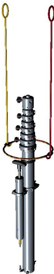
Fig. 4-1.3: grip points of the mast – vertical position
