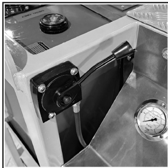
Fig. 8 – Engine throttle in lowest rpm adjustment (engine idling).
