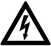
Danger due to electrical voltage
