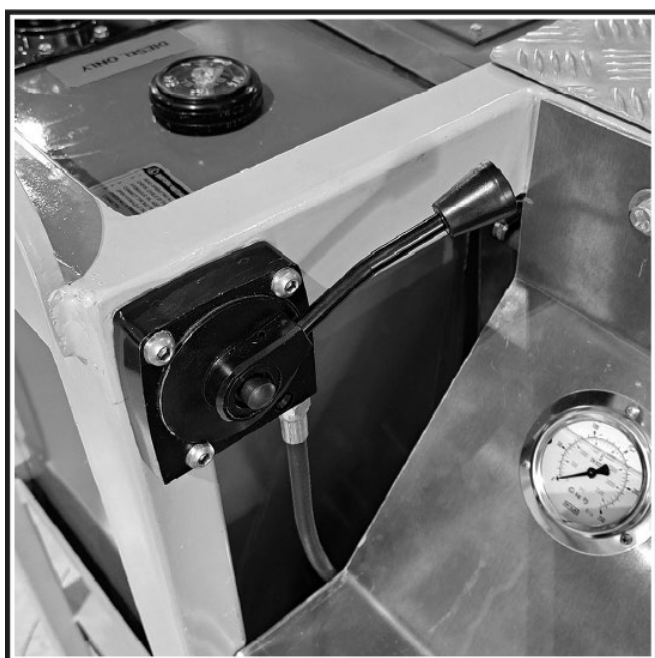
Fig. 22 – Engine throttle in lowest adjustment (engine idling)
