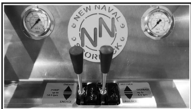
Fig. 6 – Hydraulic Controls & Pressure Gauges
