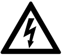
Danger due to electrical voltage
