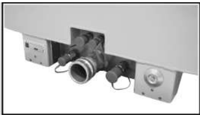
Fig. 7 – Hydraulic Inlets/Outlets & Discharge Port
