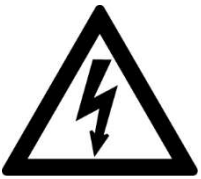
Danger due to electrical voltage
